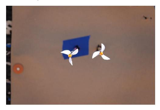
For this set and at this velocity, it took 4" feathers at 5° helical to get the broadhead under control. Part of needing this feather size is due to the low velocity.
