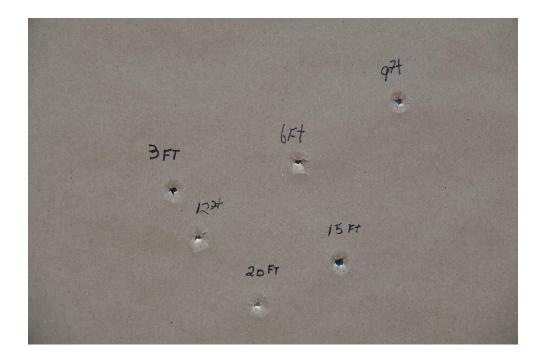
Once I have reached a level nock travel at 20ft with the bareshaft, I will compare flight and impact with both the field point and broadhead.
